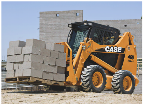
The vertical-lift 465 Series 3 is the largest skid steer offered by Case. Pilot controls for all skid steers are available from the factory in either "H" or ISO patterns.
