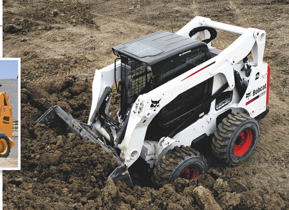
Incorporating some of the most significant design changes in the long history of Bobcat, the M-Series rolled out last summer includes the vertical-lift M650. A cab-forward design brings the operator closer to the work area and provides better overall visibility for the operator.
